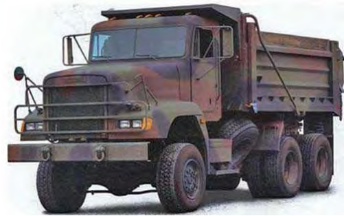
Fig. 1 M917 dump truck(Freightliner LLC) If work continues every day of the week for a mile tunnel with a 30 foot diameter, and using volume and weight standards used by the US Army, excavators would fill 44 of these trucks every minute, totaling 5 million yd 3 of dirt and stone, weighing up to 8.75 million tons.
