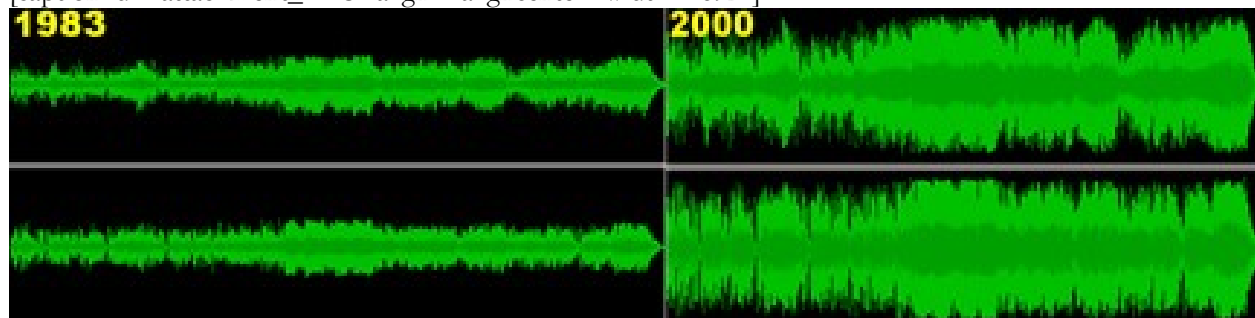
Fig. 1. The audio of The Beatles’ 1968 track ‘Something.’ On the left is the track mastered on the original 1983 CD of Abbey Road . To the right is the version mastered in 2000 for their greatest hits album 1. The 1983 version has plenty of dynamics, where the 2000 version is completely lacking in this area. Source: MK-Guitar.com[/caption]
