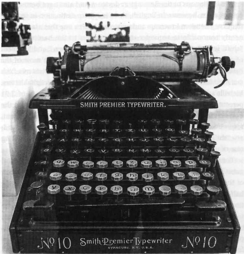
1.4 The Smith Premier double-keyboard typewriter
