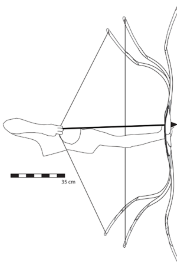
Fig. 36. Reconstruction of the approximate shape of the SBR-12 bow in unstrung, braced and drawn condition. The arrow is about 75 cm long.
