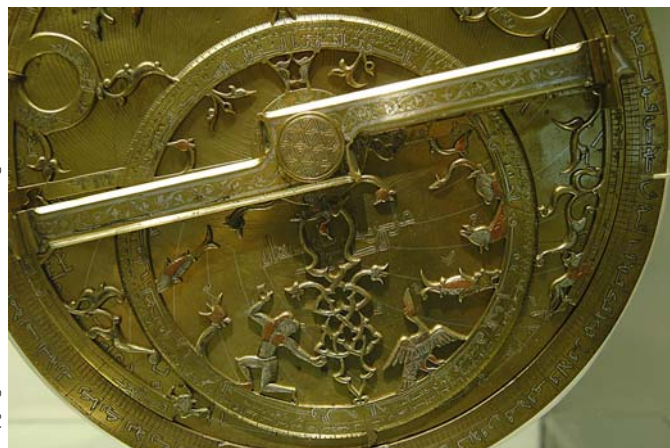
Fig. 8. Although not one of the instruments purportedly sent to China, astrolabes, like this elegantly decorated one in brass with silver inlay, made in AH 638/CE 1241 by Abd al-Karim al-Misri, exemplify the superb craftsmanship of Muslim astronomical instruments. Collection of the British Museum, Inv. no. ME OA 1855.7-9.1.
